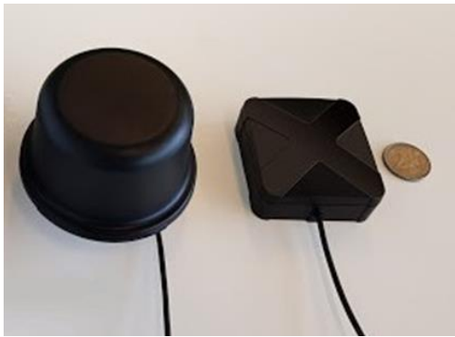
Fig. 5. GNSS antenna tested from left to right: Taoglas XAHP.50.A, Taoglas AA.200 and 2 euros coin.
